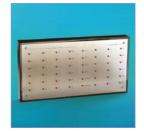
**mimic panel** – the mimic panel is usually located behind the reception desk or in a secure location. It features an array of single red LED's, each one representing a refuge point or location within the building. When a call is generated the mimic panel will display a visual indication of the call location. The mimic panel is made from 1.5 gauge stainless steel and can be custom engraved.
