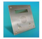
**LCD display** – the intercom display unit reports all system activity and alerts management to the location of a call within the building. The unit features a 32 character LCD display with backlight and a microphone and speaker, allowing 2 way communication between the display and the intercom point. It is manufactured from 1.5 gauge stainless steel and can be flush or desk mounted.
